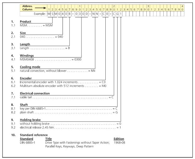
Fig. 8-3: Type code for motor MSM040B
